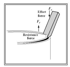
The number of times a machine multiplies the effort force is called the **mechanical advantage**. The mechanical advantage is determined using the following equations:
