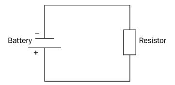
If the value of the resistor is replaced with another resistor that has a resistance of four times the initial value, how does the flow of electrons through the wire change?
